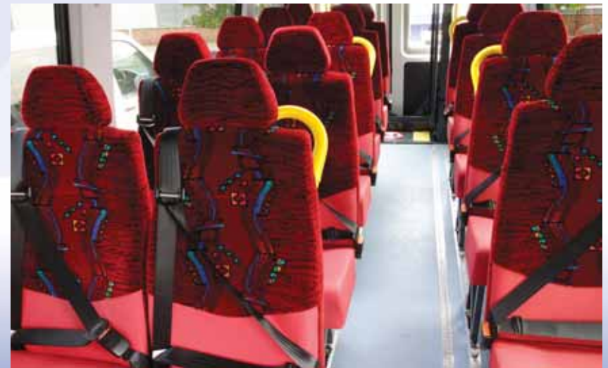
Seats with moquette and wipe clean base squab, all age seat belts, trimmed head rests and grab handles.
