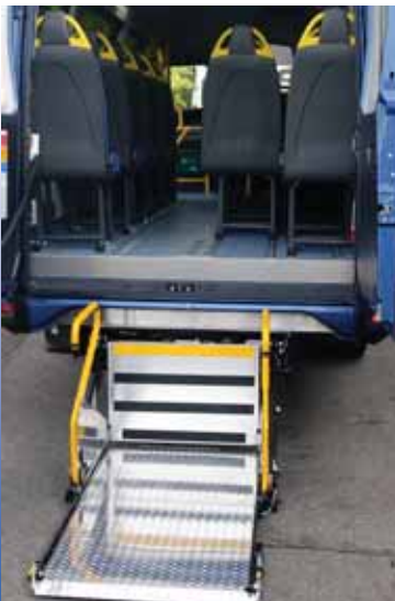
External cassette type passenger lift deployed
